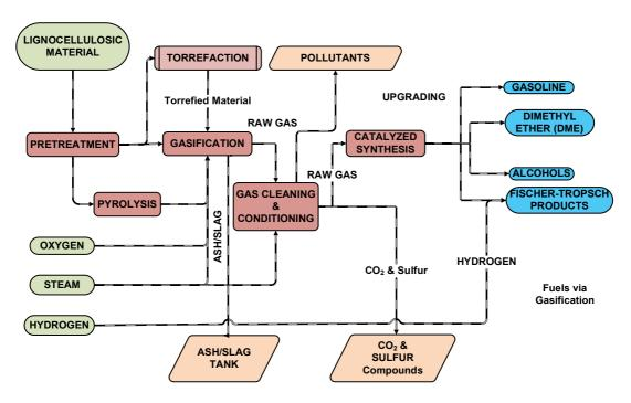
Figure 41 Fuels, industrial chemicals & hydrocarbons via biomass gasification and syntheis<sup>12</sup>
