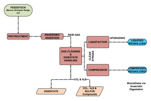
Figure 39 Simplified process flow diagram for biomethane from anaerobic digestion 104
