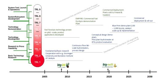
Figure 46 Technology development from basic research to commercialisation for BTG's fast pyrolysis process (courtesy Mr René Venendaal, CEO BTG)
